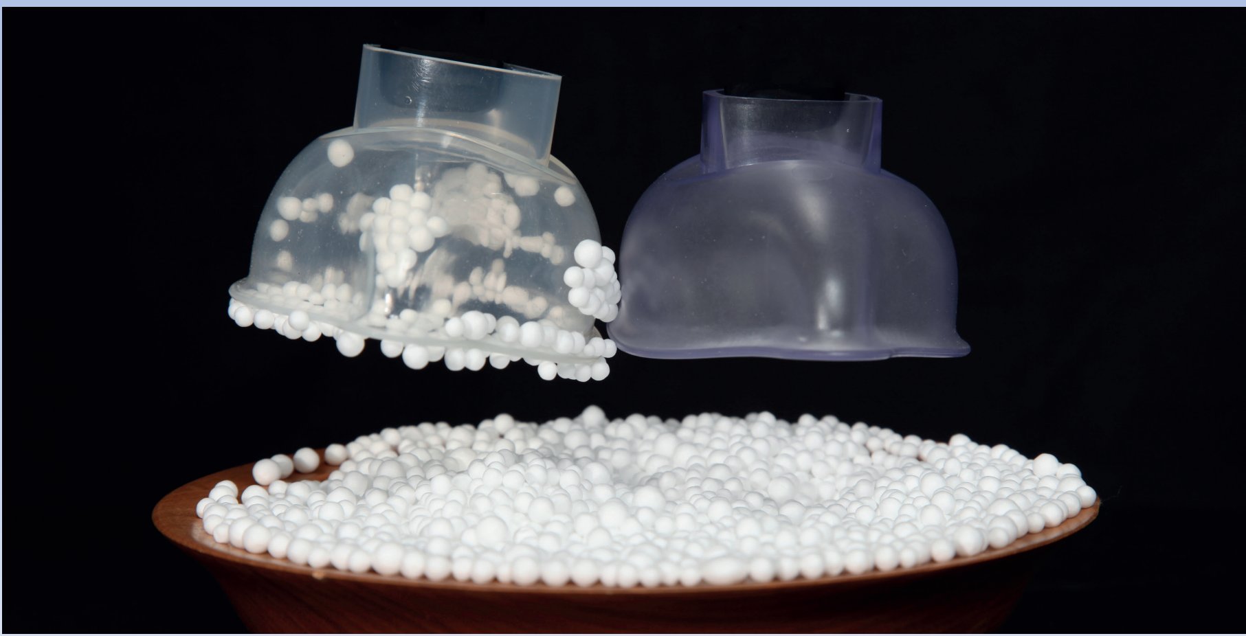
Figure 2 - Polystyrene ball test: silicone polymer (L) and new development polymer (R)
